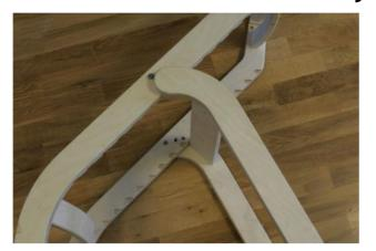
Make sure that the pivot bolt facing the floor hits the pivot hole in the back leg placed on the floor.
