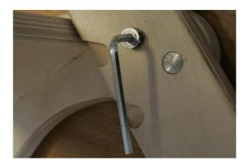
Screw in one bolt on each side and tighten it properly.
